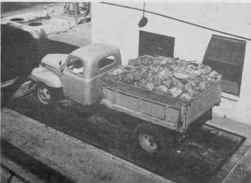
AT THE Concrete Plant, a truckload of rock is weighed on the kilogram scale. This protects both the supplier and the buyer, Lago. It is one of the few instances at Lago when metric weights are recorded. Avoirdupois weight is normally used.
